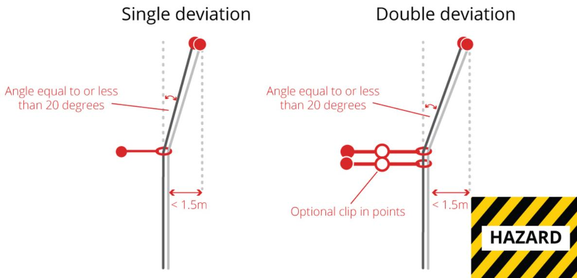
Deviation rigging examples 2 and 3 show double deviations with large distances and angles. These are used for rigging only with no requirement for technicians to pass.
